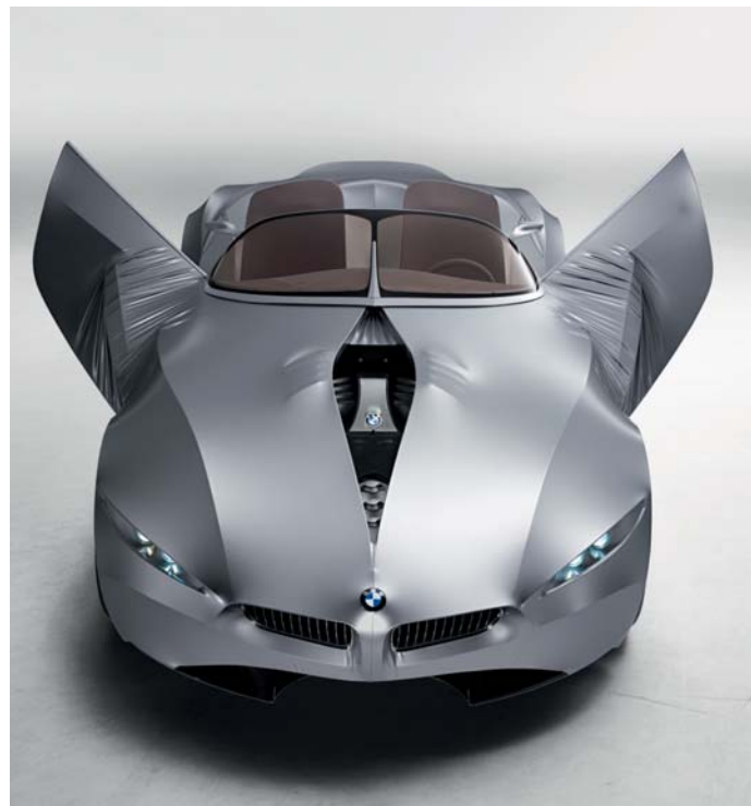
Dwight Eisenhower (left) stands in one of the first production 1953 Cadillac Eldorados at his January inauguration. BMW's GINA Light Visionary Concept vehicle (2008). An elastic skin is stretched over a frame with movable components to create a transformable appearance. GINA is the epitome of the concept car—the showcase vehicle pioneered by Harley Earl.
