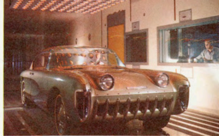
Conditions duplicating a car traveling 100 miles per hour under a midsummer sun can be produced in the Research wind tunnel.
